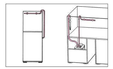
**TIP:** If you place the tubing into warm water for some time beforehand, they will become soft and possible kinks can be easily squeezed out.
