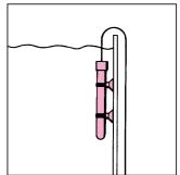
Do not install the temperature sensor near the filter outflow.
