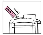
Attach the two-part tubing clamp around the installed tubing, hang into the proper position and clip into place.
