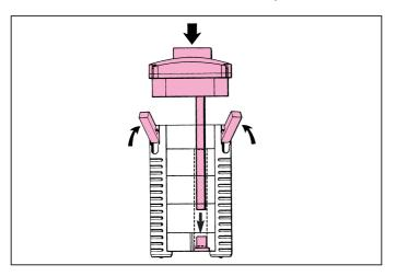
**ATTENTION:** Before the integrated double tap connector is inserted into the pump head of the filter, examine all three orings for damage and correct fitting. Lightly grease the orings with Vaseline to help installation.
