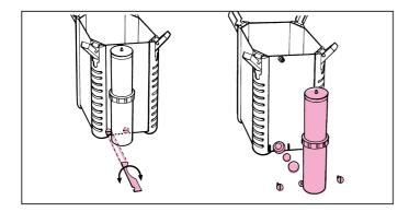
Open the locking ring of the wet/dry floater compartment in the direction indicated, remove floating control valve and carefully clean with a soft sponge.
