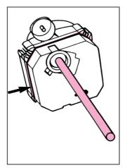
Slightly lubricate the o-ring of the output pipe and insert it firmly into the pump cover. Examine the sealing gasket on the pump head of the filter for cleanliness and proper fit.
