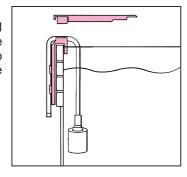
Connect the security outlet pipe and spray bar with a short piece of tubing and install in the aquarium with the help of the clip and suction cup. Close the open side of the spray bar with the enclosed end cap.
