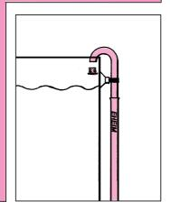
Connect the installed intake pipe and spray bar to the respective hoses.
