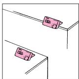
Direct the control cable from the filter canister to the thermostat. Connect the plug – you should hear it snap into place.
