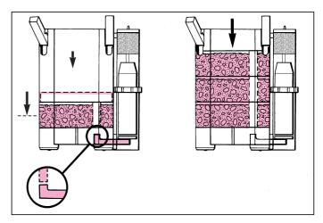
Push in the second (and third) media container in the same manner, so that the pipe openings lie on top of each other. Again lower the retractable handles for each of them and be sure that all of the media containers lie flush on top of each other. Place lattice screen.
