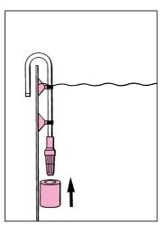
**Attention:** The foam prefilter is only to be used during the running-in period, approx. 6 - 8 weeks. Afterwards the bacteria strains in the filter media take over the biological and mechanical filtration. The foam prefilter should then be removed.
