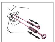
Pay attention to the proper fit of the shaft bushings, pump cover and sealing ring. Then lock the pump with the sealing ring.
