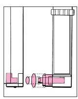
Place the first media container back into the canister in such a manner that the flow-through opening sits above the connection outlet which communicates with the wet/dry floater compartment. Press the container down to the support frame in order to guarantee a good seal with the filter canister.
