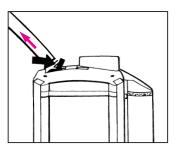
Swing the locking clamp upwards and then remove the double tap connector from the pump head. Extract the filter out of the cabinet by using the recessed handles.
