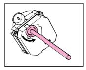
Thoroughly clean pump parts, impeller chamber and lubrication channel with the EHEIM cleaning set (order no. 4009580.)
